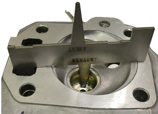
The spark plug insert must show a clearance to the CPO gauge, which must be flush on the cylinder face
