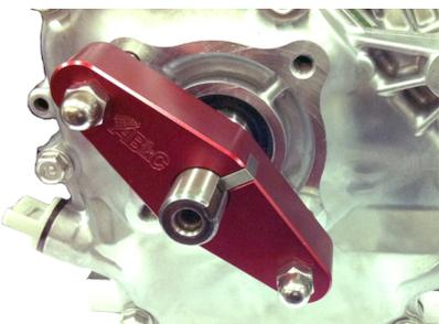
If the output shaft keyway and throw of the crankshaft are aligned then the ABkC-marked location tool can be used to assist with the setting. For accuracy, the crankshaft must be
