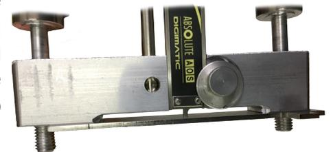
Using the CPO gauge to zero a caliper prior to its use for stroke and deck height readings
