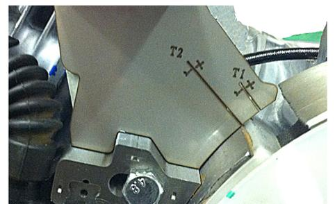
rotated against the location tool in a clockwise direction (flywheel side) before the reading is observed on the template tool. The standard and unmodified fan must be used, with all fins in place.
